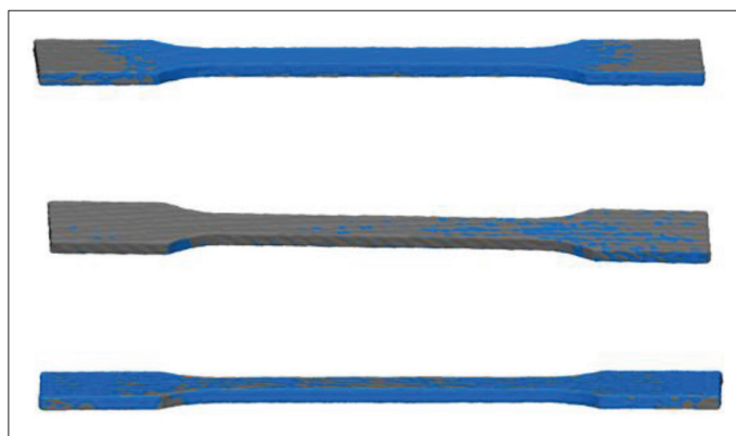
Figure S16. PA12 control and HPO samples pre-aligned before the mesh analysis.
