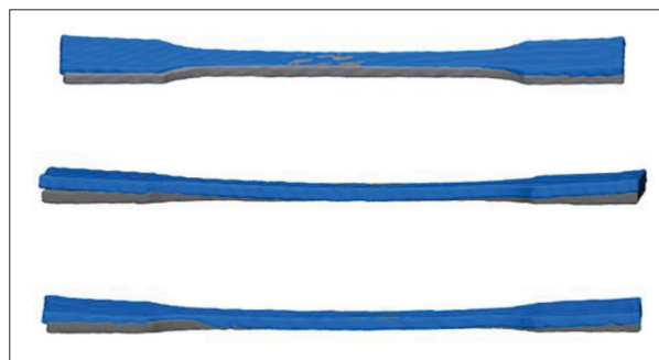
Figure S12. MED610 control and AU121 samples prealigned before the mesh analysis.
