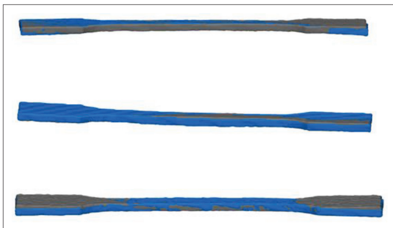
Figure S32. VERO control and AU121 samples prealigned before the mesh analysis.
