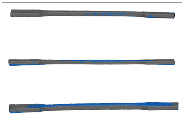
Figure S28. Surgical Guide resin control and AU134 samples prealigned before the mesh analysis.
