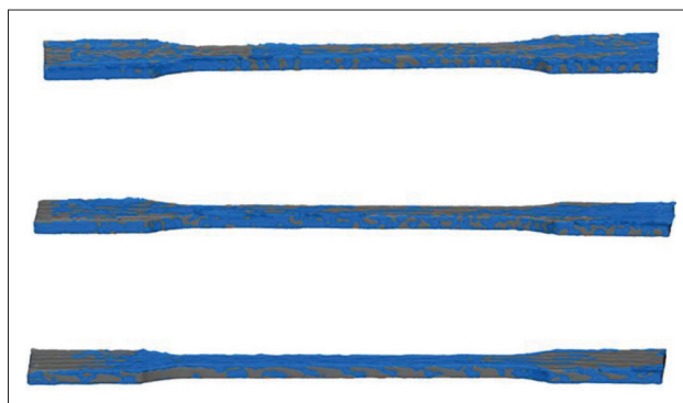
Figure S2. Acrylonitrile butadiene styrene (ABS) control and HPO samples prealigned before the mesh analysis.
