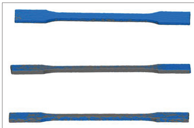
Figure S20. PA12 control and AU134 samples prealigned before the mesh analysis.
