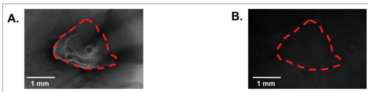
Figure S2. Bioink does not demonstrate autofluorescence or activate calcein AM. (A and B) Bioink composed of 1% sodium alginate and 6% gelatin without tumor cells was printed onto a 6-well plate. An image of bioink with calcein AM dye added was taken (A) without fluorescence and (B) under fluorescein-5-isothiocyanate (FITC) laser. The bioink did not autofluorescence or fluoresce with calcein AM.
