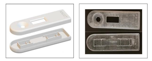
Figure S2. CAD of the housing unit design 3D printed housing unit for the
