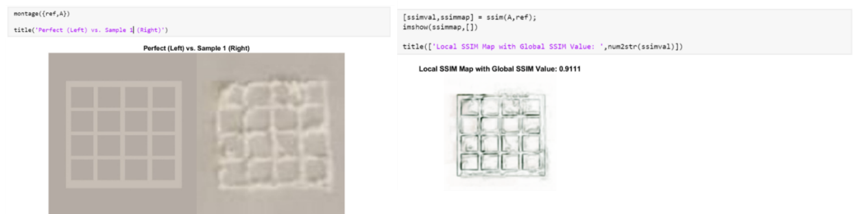
Figure S3. Data obtained from the image processing analysis to find the best ratio of bioceramics that are imbued in the biopolymer-base. Also, an example of how the MATLAB code is working, where two images are compared, and we get a convergence of both pictures that gives us a mathematical value to process in a statistical model.
