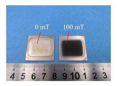
Figure S4. The effect of magnetic field on coating preparation.
