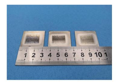
Figure S1. Photograph of the coating obtained when GO is agglomerated in the plating bath.
