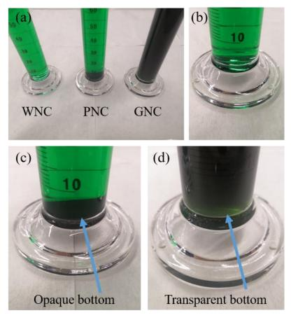
**Figure S3.** Sedimentation of plating bath standing for 1 hour. (**A**) Equal amounts of different types of plating bath. (**B**) Watts nickel bath. (**C**) Plating bath used to prepare PNC. (**D**) composite plating bath used to prepare GNC.
