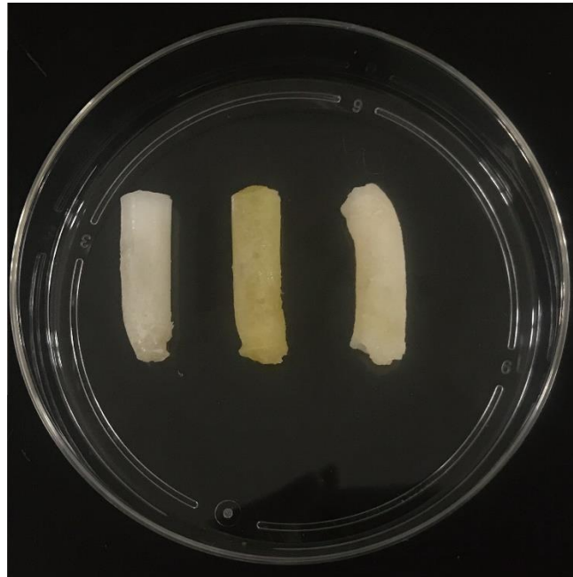
Figure S1. PVA/dECM hydrogel with different treatment. From left to right: after being photocrosslinked, after being soaked sodium hydroxide, and after being soaked in calcium chloride.
