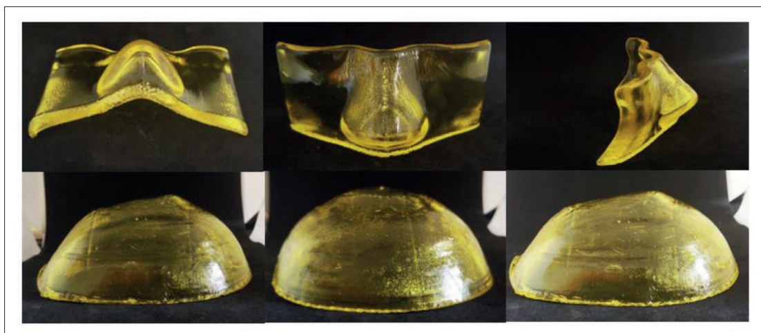
Figure S5. Boluses for head radiotherapy were printed using the gel. The top row shows the boluses that can be used for the nose, and the bottom row shows the boluses that can be used for the top of the skull.
